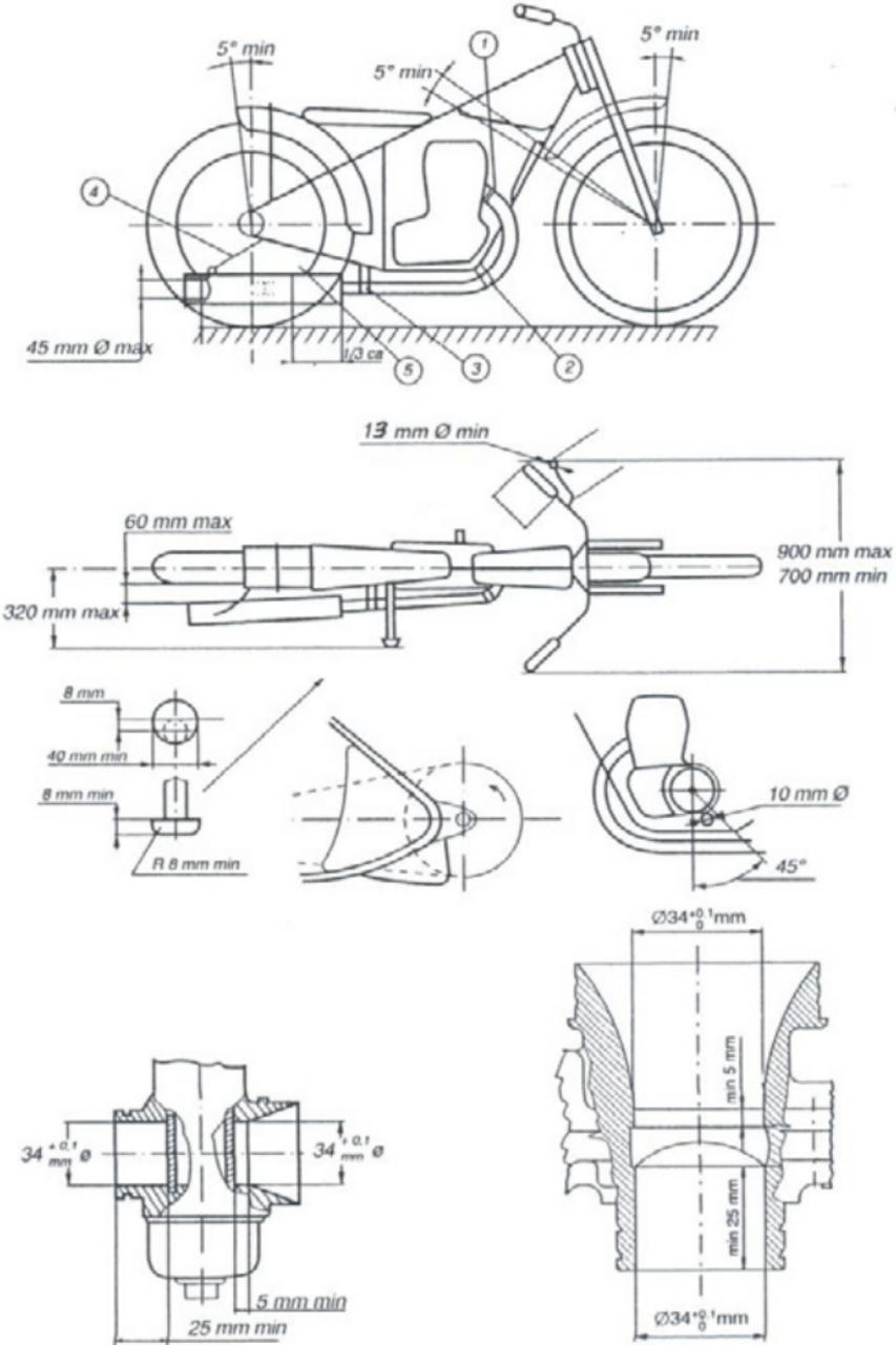
The outer edge of the right footrest must be a minimum 40mm in diameter and 8mm thick with a minimum 8mm outer edge radius.
